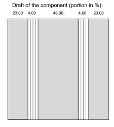
The inhomogeneous layer consists of two zones (A, B). The portion is given in %.
